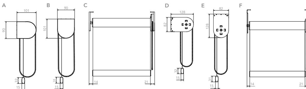
Uses System 45®+ brackets and System 45® extension brackets
